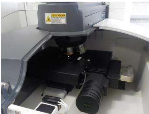
Microscopio drx raman thermoscientific. Foto: Axel Olay
